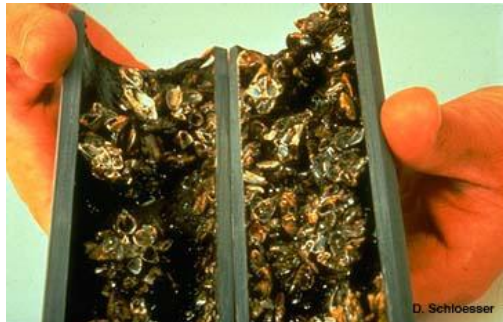
Picture 3. Zebra mussels blocking a pipe section (source: www.nyis.info )
