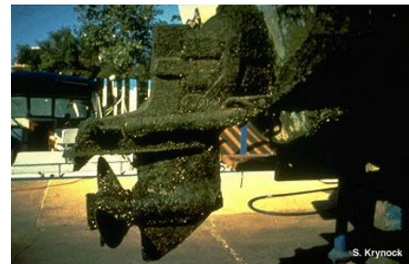
Picture 4. Zebra mussels on a boat engine (source: www.protectyourwaters.net )
